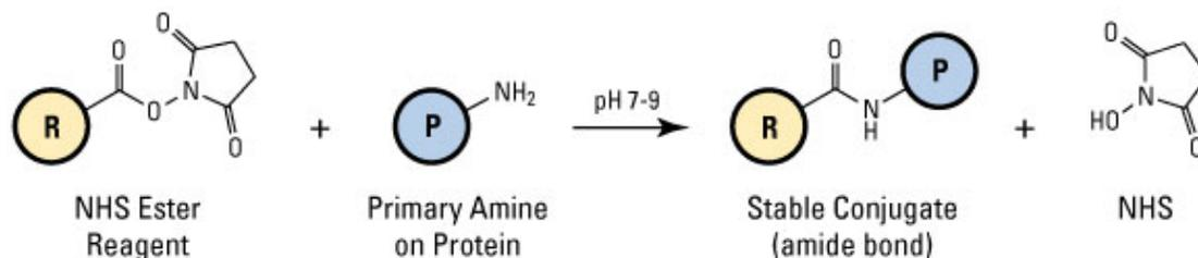
NHS ester reaction scheme for chemical conjugation to a primary amine. R represents a labeling reagent or one end of a crosslinker having the NHS ester reactive group; P represents a protein or other molecule that contains the target functional group (i.e., primary amine).<sup>1</sup>
